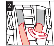
Store splitter plate by pushing it through one opening and out the other.
